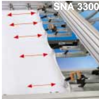
Automatic sensing, straightening, and tensioning of the comforter bag at rear of system
