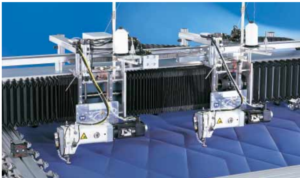
Quilting systems with double heads for increased efficiency
