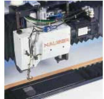
Heavy-duty sewing head for heavy / thick materials
