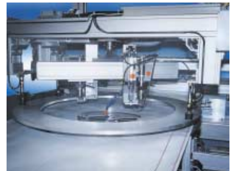
Cutting with ultrasound
