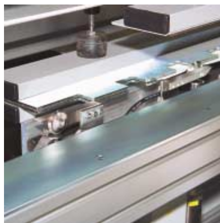
Cross-cutting with ultrasound
