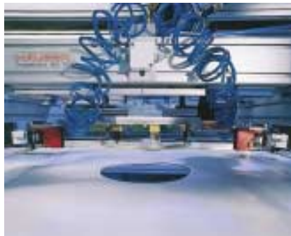
Cross-cutting with ultrasound
