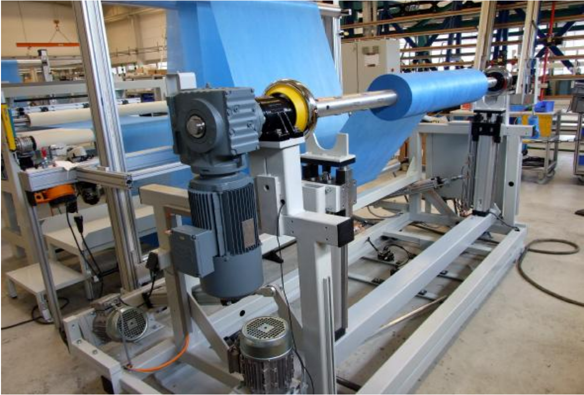
Unwinding unit driven in the center with inserting device for the material rolls
